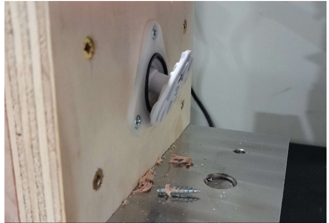
Figure 9 - Shear failure of 8G screw
