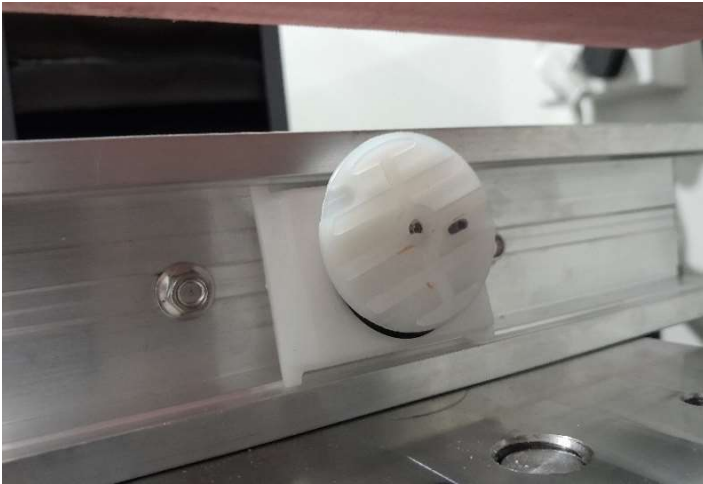
Figure 8 - Shear failure of 8G screw
