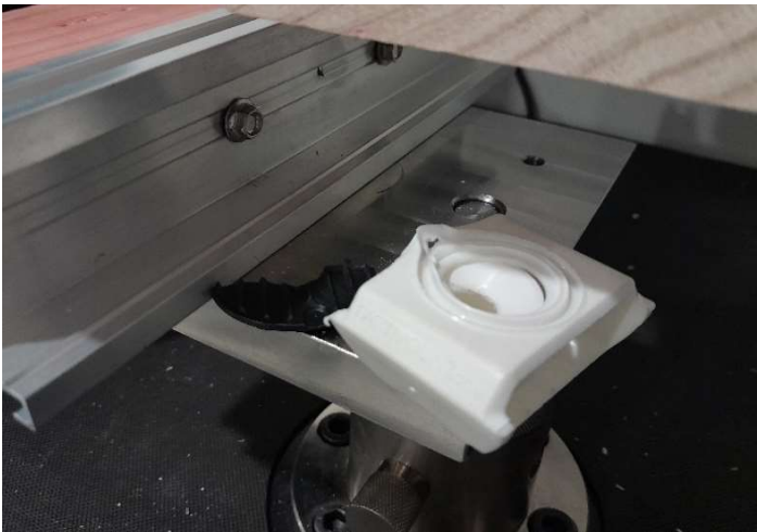
Figure 10 - Combined shear failure of the SL-FB-FR and SL-M18-FR clips
