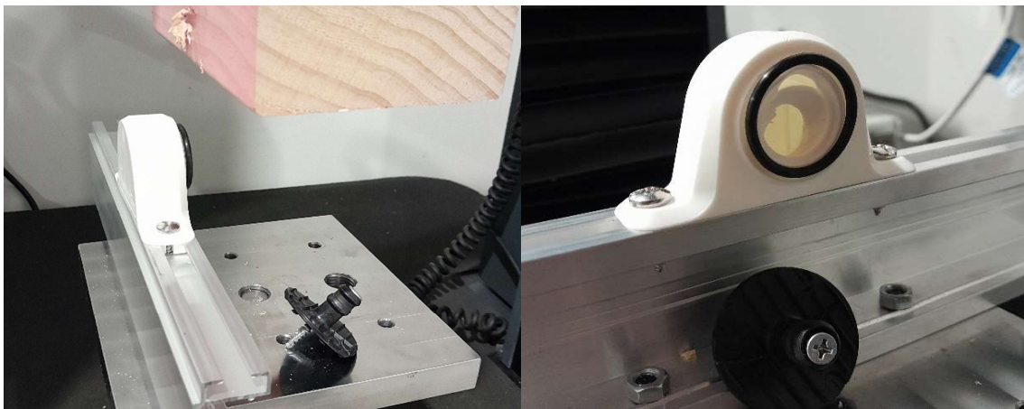
Figure 10 - Pull-out of 8G screw from timber substrate
