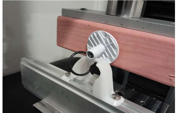
Figure 9 - Fracture of female clip housing
