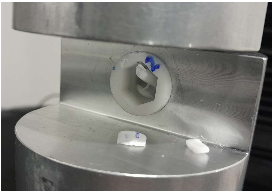
Figure 7 - Fracture of female clip housing
