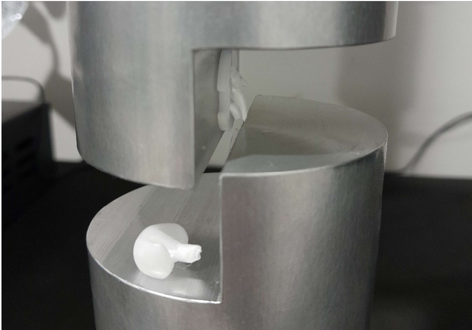
Figure 6 - Fracture of female clip housing
